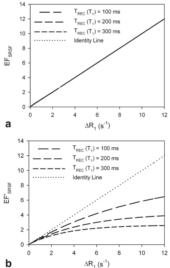
FIG. 4. SRSF enhancement indices simulated by using different  $T_1$ -weighted  $T_{\text{REC}}$ , where (a)  $EF_{\text{SRSF}}$  and (b)  $EF'_{\text{SRSF}}$  (proton density-weighted  $T_{\text{REC}} = 100$  ms and native  $T_1 = 1300$  ms were assumed).
