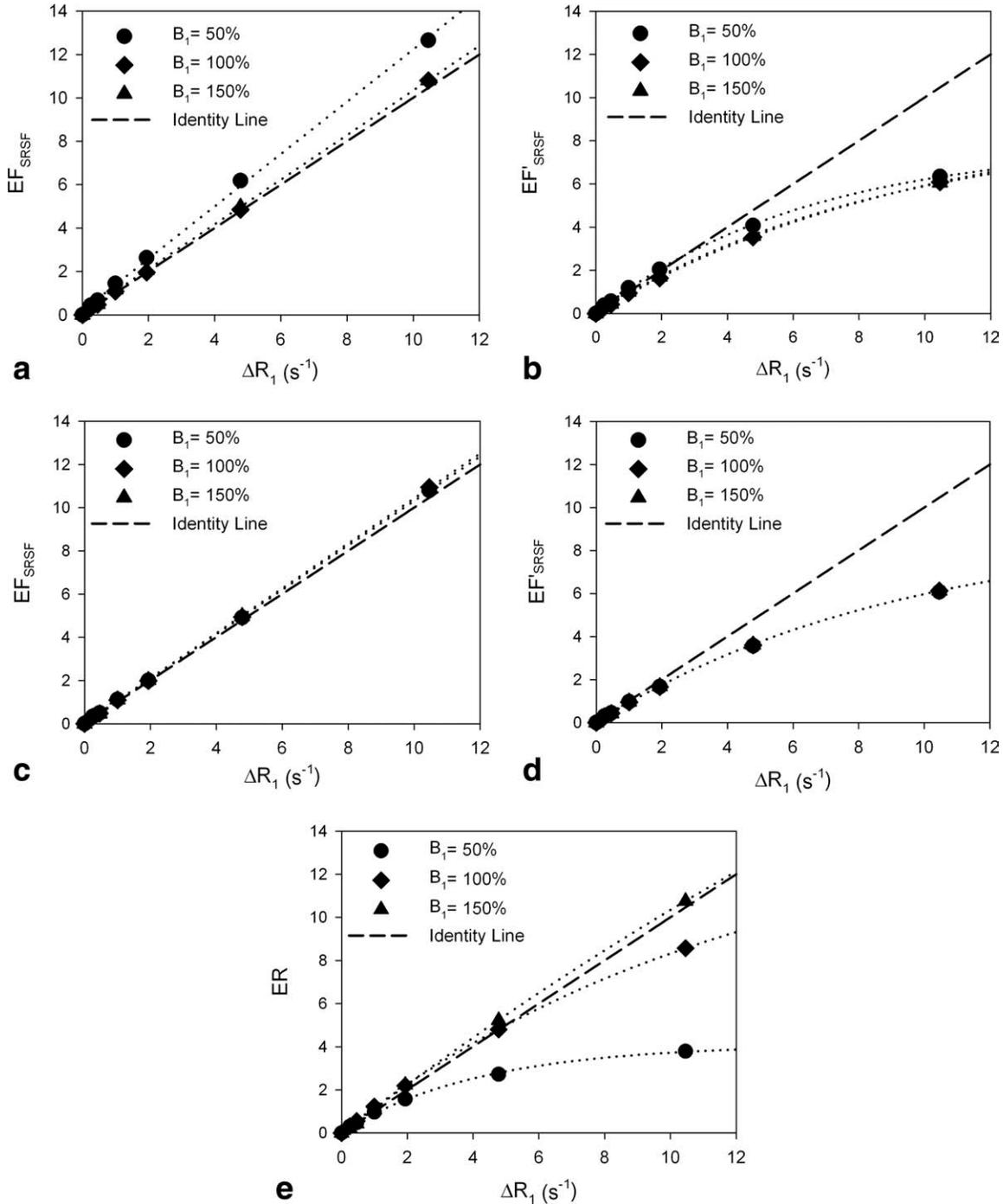
FIG. 6. The effect of  $B_1$  transmission-field inhomogeneity on the enhancement indices using two different pulse sequences, where (a)  $EF_{SRSF}$  using Hoffmann's SRSF, (b)  $EF'_{SRSF}$  using Hoffmann's SRSF, (c)  $EF_{SRSF}$  using SRSF with an effective  $90^\circ$  saturation pulse, (d)  $EF'_{SRSF}$  using SRSF with an effective  $90^\circ$  saturation pulse, and (e) ER using FLASH. The dotted lines are the fitted lines of the plotted enhancement indices.
