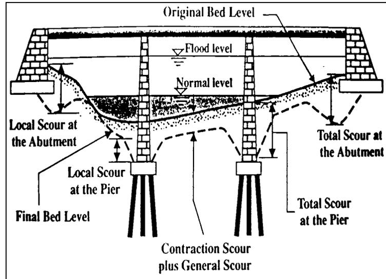
Figure 1. Types of scour occurred at a bridge (Melville and Coleman, 1999).
