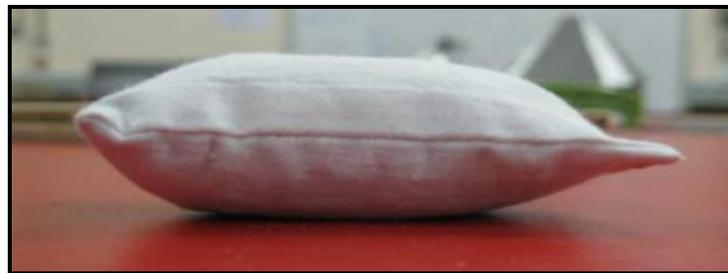
**Figure 4.** Geobag filled with crushed concrete.
