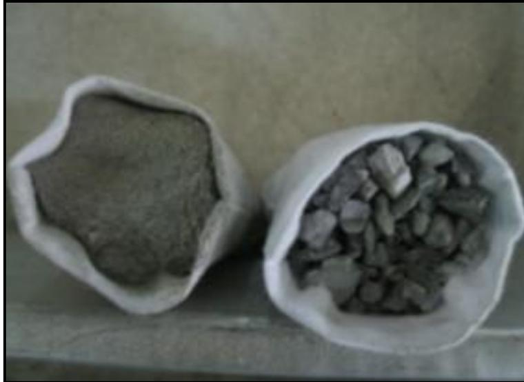
**Figure 3.** Abandoned concrete and crushed concrete.
