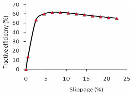
Fig. 7. Effects of slippage on the tractive efficiency
