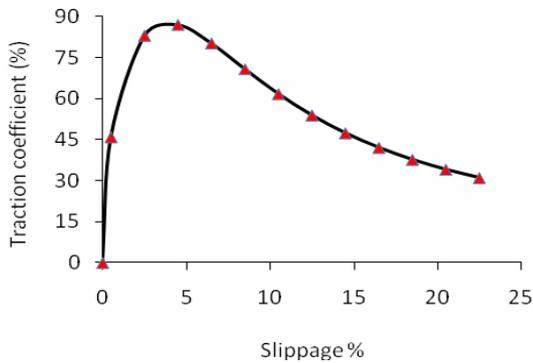
Fig. 8. Effects of slippage on the traction coefficient
