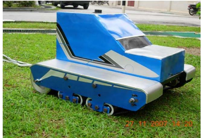
Fig. 6. Developed prototype of air-cushion track vehicle [9]
