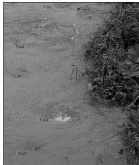
Figure 2: Momentum transfer characterized by series of vortices at the interface region of main channel and flood plain [2].
