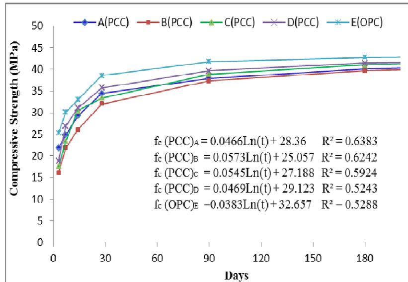
Fig. 1. Comparison of compressive strength gain with age of concrete made with various cement for 41.37 MPa.
