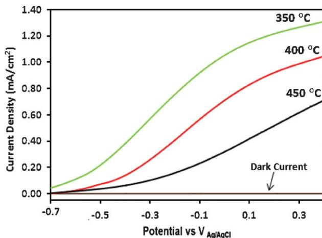
Fig. 9.  $J$ - $V$  curves for the greenockite (CdS) thin film electrodes deposited from **1** in pyridine measured under simulated AM 1.5 sunlight in aqueous 0.1M  $\text{Na}_2\text{SO}_3$  solution as an electrolyte.
