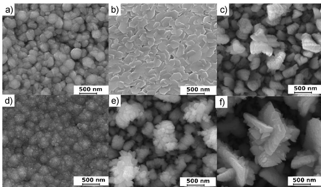
Fig. 6. SEM images of greenockite (CdS) thin films deposited from **1** on FTO (a–c) and soda glass (d–f) at 350, 400, and 450 °C in toluene solution, respectively.
