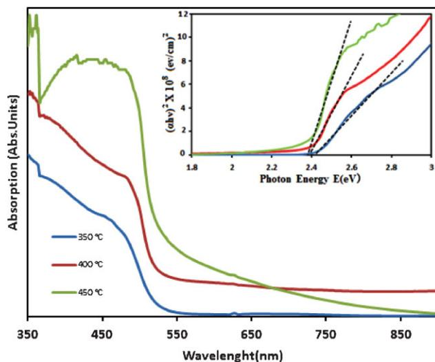
Fig. 8. Optical absorption spectrum of greenockite (CdS) thin films deposited from precursor **1**. Inset: Tauc plot showing the estimated optical band gap of 2.4.
