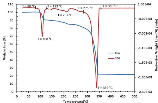
Fig. 3. TGA/DTG plots showing losses in mass with increase in temperature for precursor **1**.
