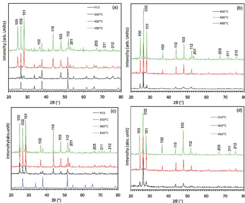
Fig. 4. XRD patterns of greenockite CdS thin films deposited from **1** on substrates (a) FTO, (b) soda glass using pyridine; (c) FTO, (d) soda glass via THF solutions at 350, 400, and 450 °C, respectively.
