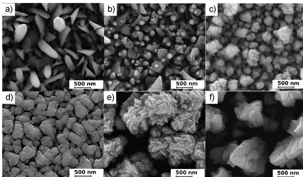
Fig. 7. SEM images of greenockite (CdS) thin films deposited from **1** on FTO (a–c) and soda glass (d–f) at 350, 400, and 450 °C from THF solution, respectively.
