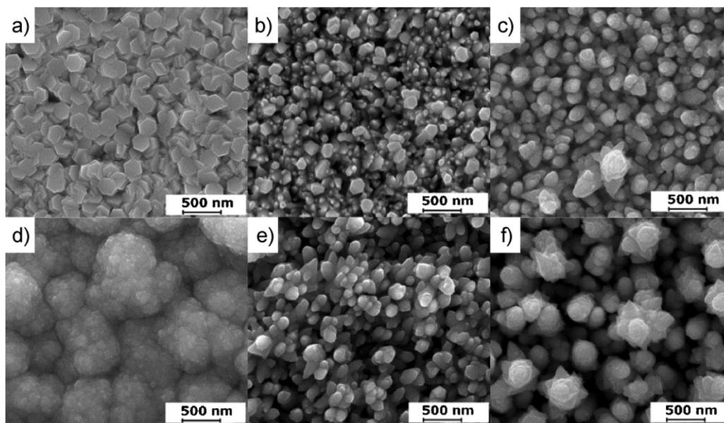
Fig. 5. SEM images of greenockite(CdS) thin films deposited from **1** on FTO (a–c) and soda glass (d–f) at 350, 400, and 450 °C in pyridine solution, respectively.
