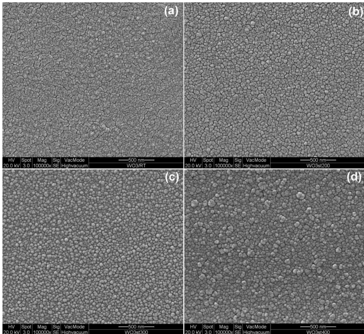
2 Images (SEM) of  $\text{WO}_3$  films deposited at *a* room temperature, *b* 200°C, *c* 300°C and *d* 400°C
