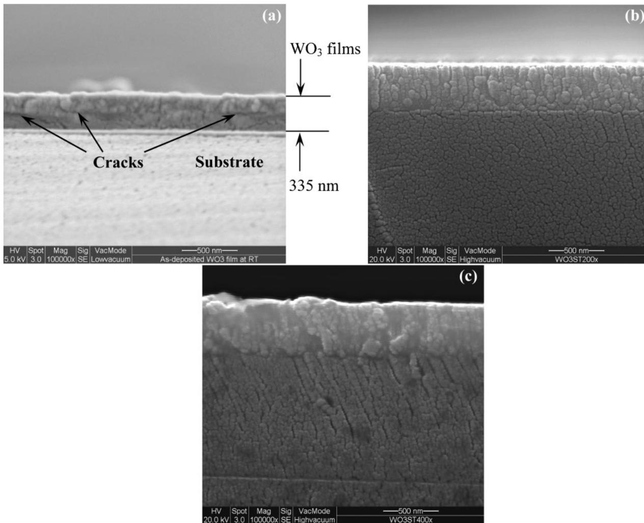
3 Cross-sectional views (SEM) of WO<sub>3</sub> films deposited at a room temperature, b 200°C and c 400°C
