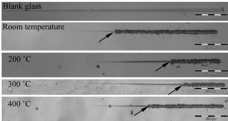
4 Optical micrographs of scratches made under progressively increasing load on blank glass and WO<sub>3</sub> films deposited at different temperatures
