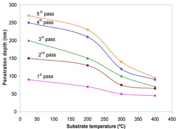
6 Total depth of penetration after each wear pass for WO<sub>3</sub> films deposited at different temperatures
