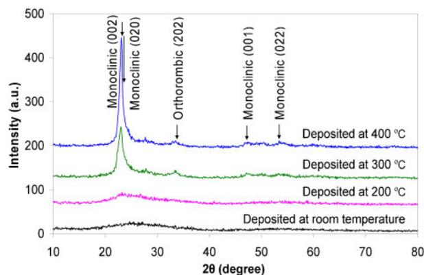
1 X-ray diffraction patterns of  $\text{WO}_3$  films deposited at different substrate temperatures
