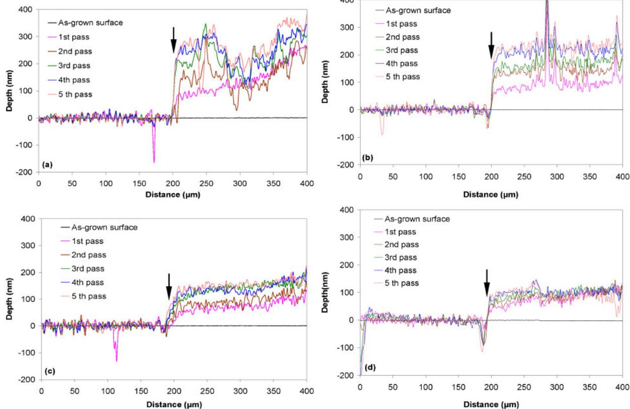
5 Wear tests for WO<sub>3</sub> films deposited at a room temperature, b 200°C, c 300°C and d 400°C
