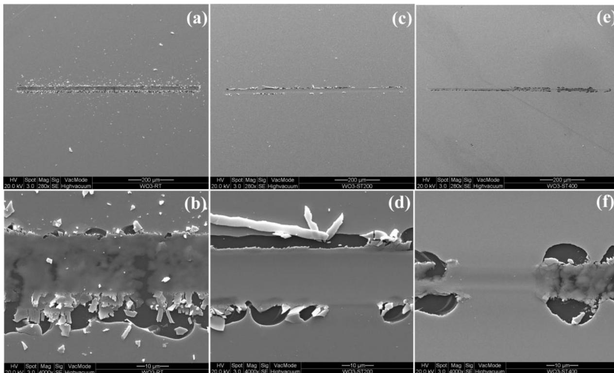
7 Image (SEM) of wear scars on WO<sub>3</sub> films deposited at a, b room temperature, c, d 200°C and e, f 400°C after five passes
