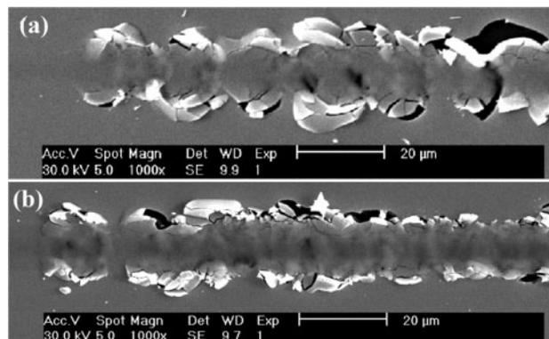
**8 Images (SEM) for scratches on WO<sub>3</sub> films deposited at a room temperature and b 400°C (× 1000)**
