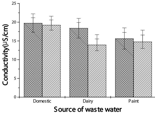
**Figure 5.** Conductivity before and after treatment. : Untreated : Treated
