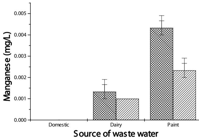
**Figure 8.** Concentration of Manganese before and after treatment.
