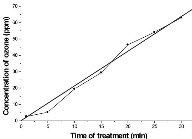
**Figure 2.** Concentration of ozone dissolved in waste water after different treatment times. — Linear fit
