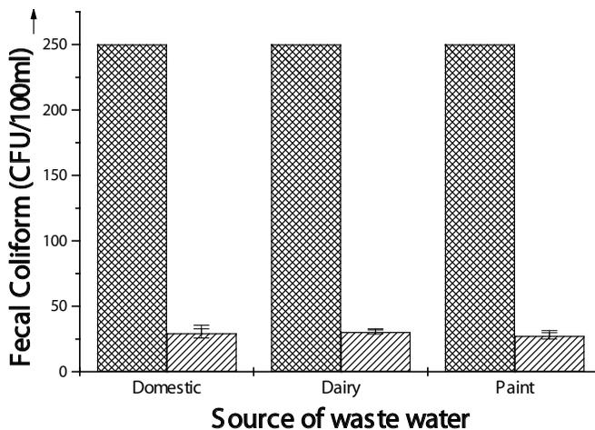
**Figure 10.** Fecal coliform count before and after treatment.
