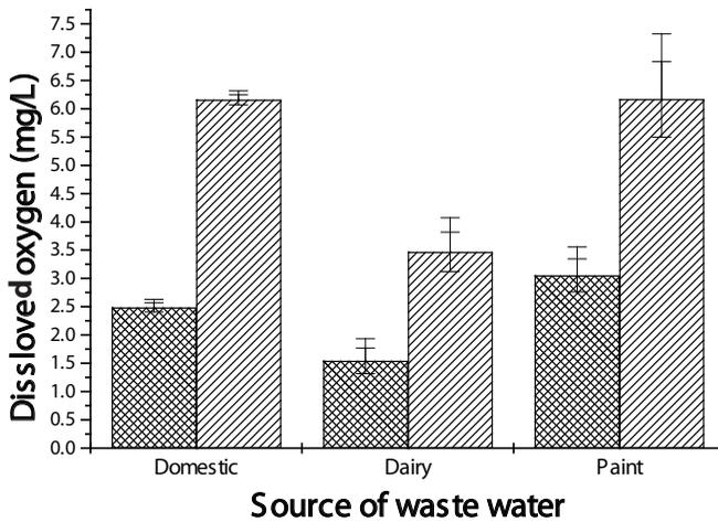
**Figure 6.** Concentration of DO before and after treatment. : Untreated : Treated
