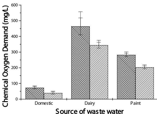
**Figure 7.** COD before and after treatment.
