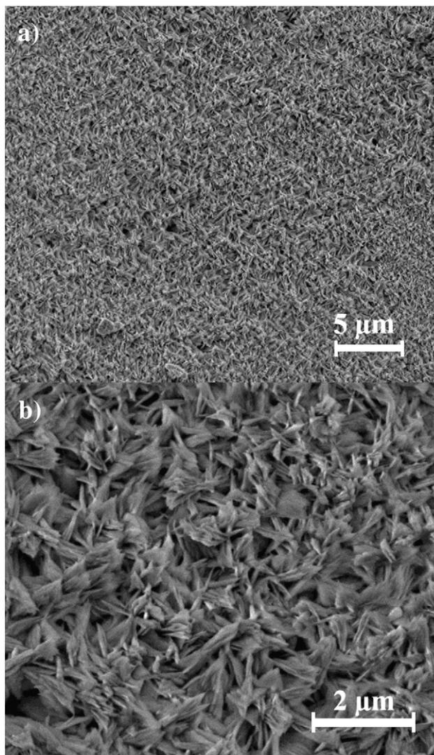
Fig. 1. FESEM micrographs of copper oxide nanoflakes. (a) Lower magnification, (b) higher magnification.
