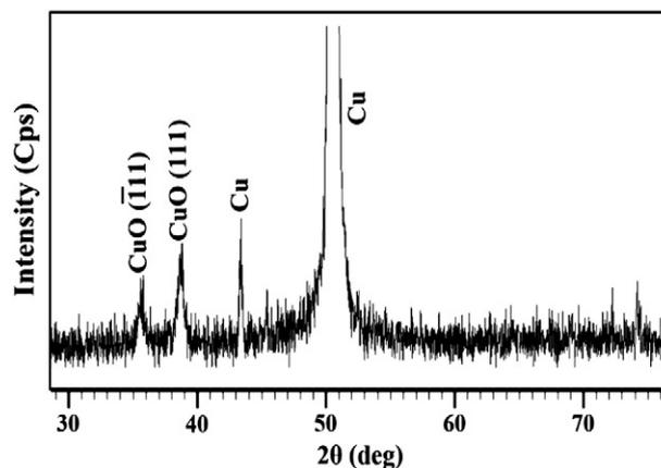
Fig. 2. XRD pattern of copper oxide nanoflakes.
