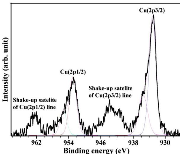
Fig. 3. The XPS spectrum of the Cu(2p) core level of the copper oxide nanoflakes (thick line). The fitted curves are shown under the spectrum (thin line).
