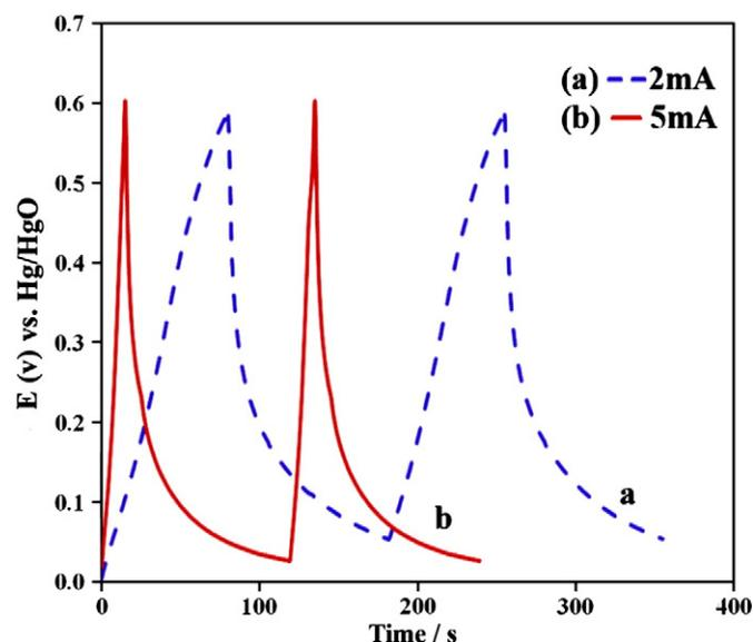
Fig. 5. Galvanostatic charge–discharge of copper oxide nanoflakes with different currents: (a) 2 mA, (b) 5 mA.
