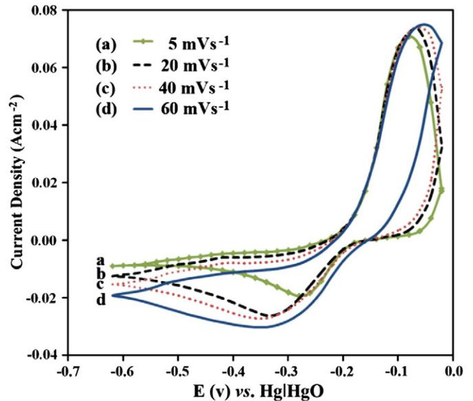
Fig. 4. Cyclic voltammograms of the as-prepared copper oxide nanoflakes electrode in 1 M KOH electrolyte.
