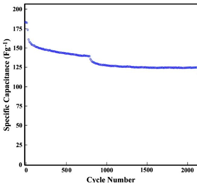
Fig. 6. Cyclability test of copper oxide nanoflakes at a current density of  $2 \text{ mA cm}^{-2}$ .
