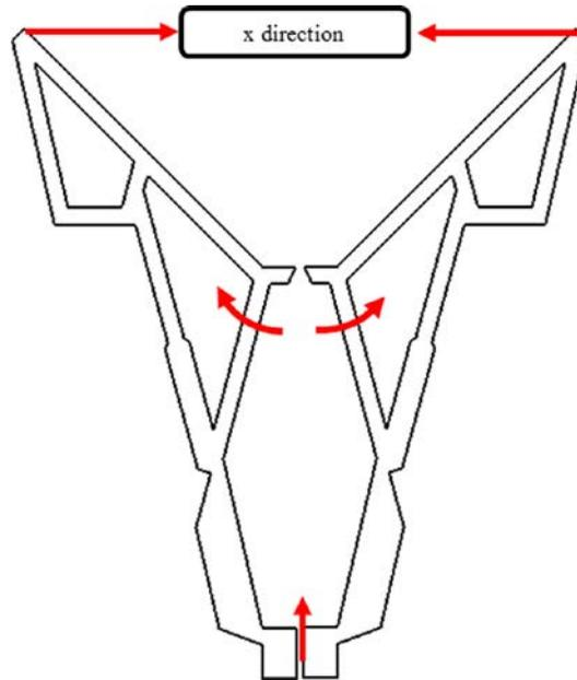
Figure 10 Optimal design for the finger mechanism obtained by FEM iterative method
