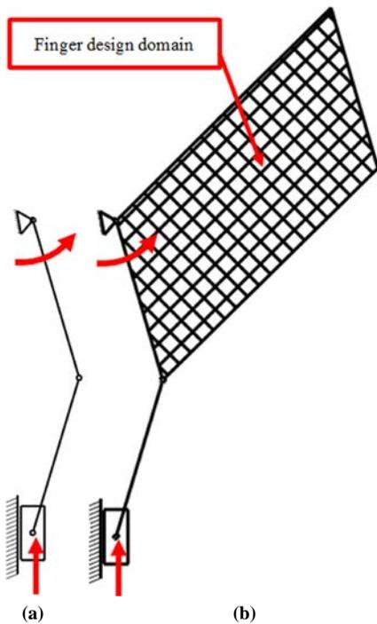
**Figure 7** Initial gripper structure with all optimization parameters for FEM optimization procedure
