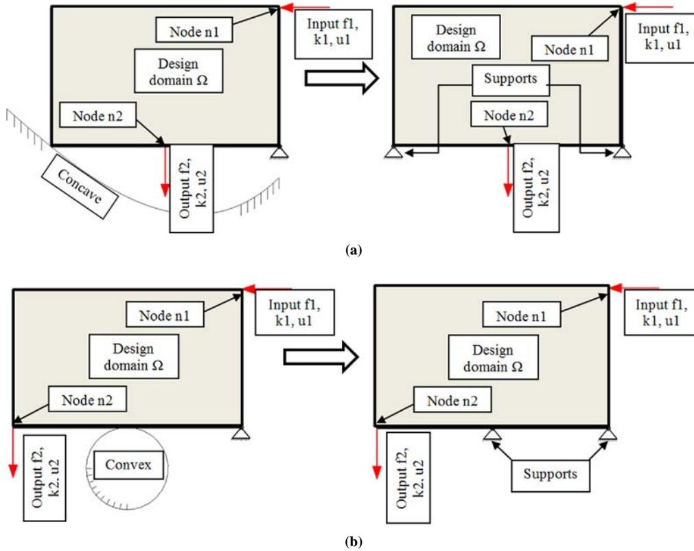
**Figure 3** Design domain discretization by density elements; optimization variable is element density (a) and possible topology structure for a compliant mechanism (b)
