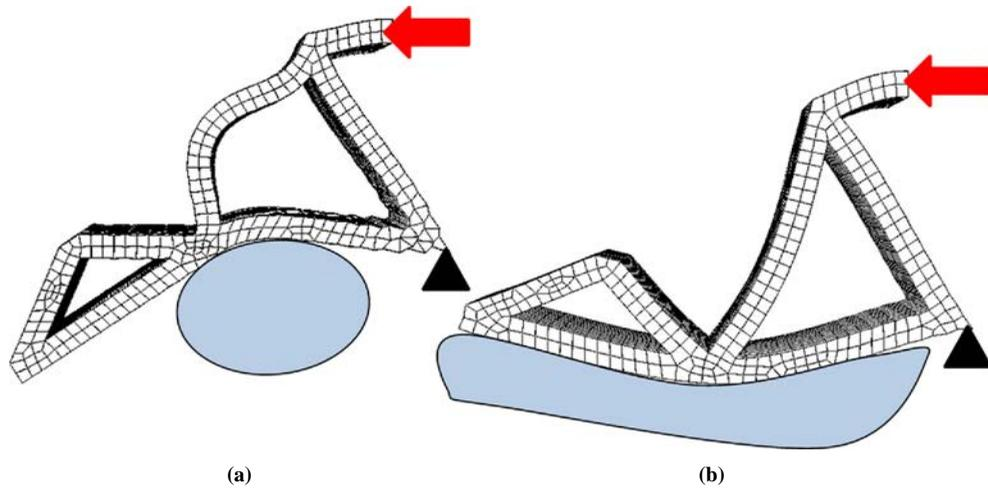
**Figure 6** Input mechanism for on finger as (a) slider crank mechanism and (b) finger design domain
