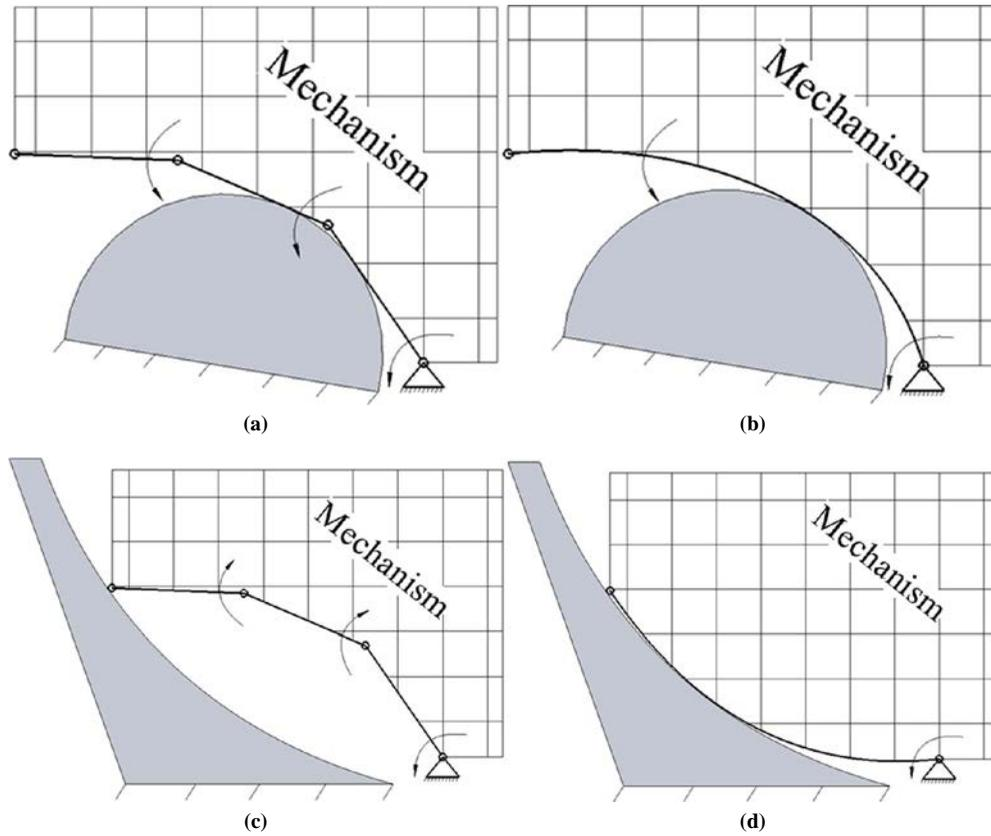
**Notes:** (a) Rigid body finger behavior for convex grasping shape; (b) compliant finger behavior for convex grasping shape; (c) rigid body finger behavior for concave grasping shape; (d) compliant finger behavior for concave grasping shape
