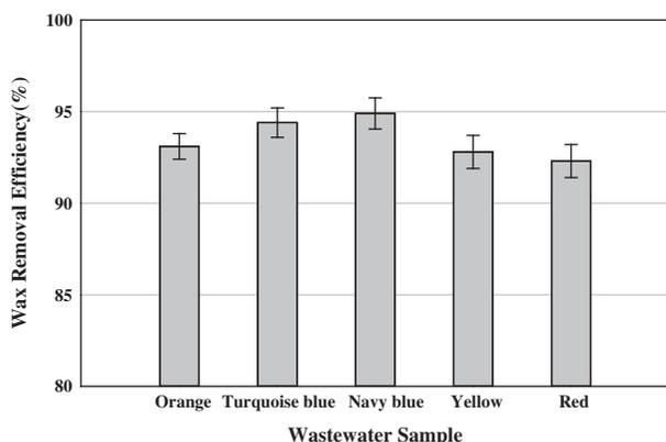
Fig. 2. Wax removal efficiency in single dye samples.
