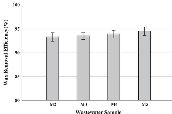
Fig. 3. Wax removal efficiency in mixture dyes samples.
