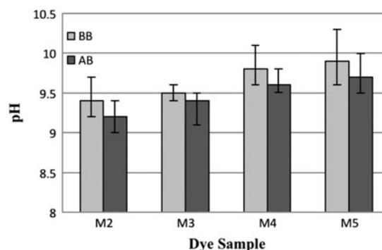
Fig. 9. pH removal efficiency in mixture dye wastewater samples.
